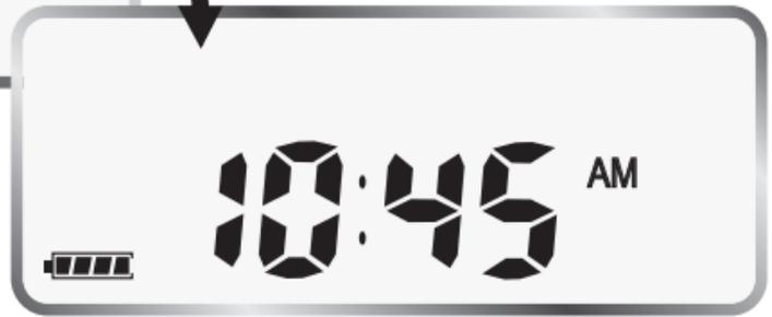
With the dial in the **OFF** position the current time will be displayed and will alternate to then show **OFF**. (continual alternation)
