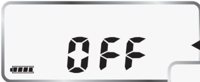
**OFF Mode** - Turning the dial to the **OFF** position from any other position will stop the **MANUAL** or **AUTO** Watering in 5 seconds. (screen alternates)
