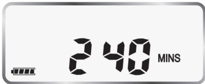
Rotate the dial to '**HOW LONG**' and select from 1 minute to 360 minutes using the **+** and **-** buttons.
