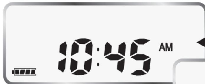
**MANUAL Mode** - Operates manually with 360 minutes adjustable clock count down.
