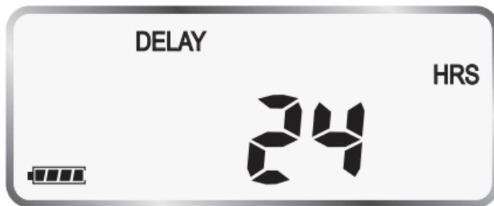
This function delays the nominated start time. Ideal for delaying watering after heavy rain.
