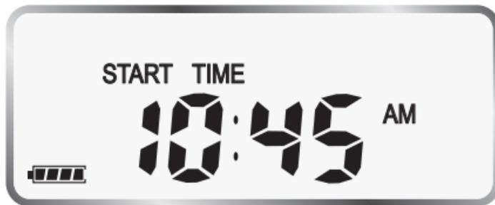
Rotate the dial to **'START TIME'** and set the start time for automatic watering.
