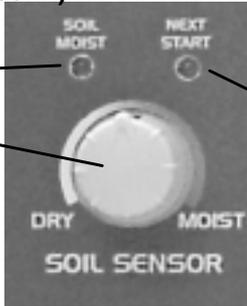
"Next Start" amber light will come on when watering is required. The controller will then run the next scheduled watering cycle.
