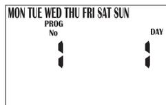
To turn Monday off press the **-** button. To turn it back on press the **+** button. To advance to the next day and set it use the **▶** button, the display will then flash Tue and Day 2. Use **+** or **-** to turn days ON or OFF and advance to the next day using **▶**. Remember to set all 7 days ON or OFF.
