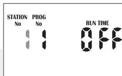
**NOTE:** This means that station 1 of program 1 has no run time programmed in it. The controller has permanent memory so when the device is first used there will be no run times set. Unlike other controllers, when there is a power failure, even if the battery is not installed, the programmed values will be restored to the unit.
