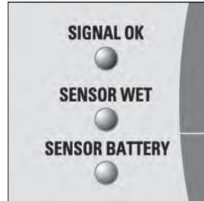
**NOTE:** *When the batteries in the rain gauge go flat and are replaced, it is important to re-set the controller, to allow the controller and rain gauge to communicate. In this instance it is important to note that when you install the Rain Gauge, ensure it is in a convenient location to access for battery replacement.*
