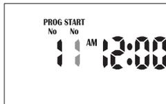
Use **+** or **-** to change the “Start No” if required, otherwise press **▶** and the “hour” will flash. Use **+** or **-** to adjust if required.
