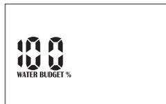
This means that the run times are set to 100%, i.e. if station 1 is set to 10 minutes then it will run for 10 minutes. Should however the value change to say 50% then instead of running for 10 minutes station 1 would now run for 50% of 10 minutes, i.e. 5 minutes.
