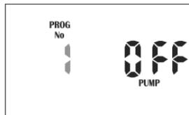
is now flashing. Press the button to turn Pump No.2 ON or press the button to turn Pump No.2 OFF for that particular number.
