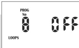
To enable the looping program press the **+** button, the display will show “ON”.
