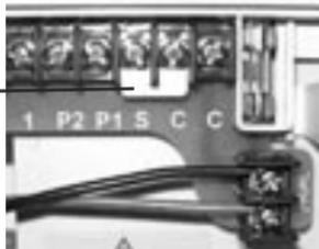
Replace with the two wires from the rain sensor into these terminals, polarity NOT required. Move the rain sensor switch on the fascia to “ON”.
