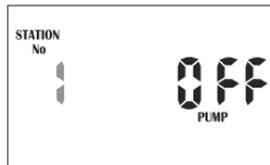
This means that pump will not turn on when station No 1 is running. To turn a pump ON or OFF for a particular station
