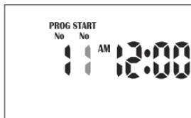
Use **+** or **-** to change the “Start No” if required, otherwise press **▶** and the “hour” will flash. Use **+** or **-** to adjust if required.
