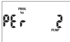
This means we are in the pump per program menu for Pump No.2 (master valve No.2). Press the button to enter this menu option. Program 1 will now be flashing.
